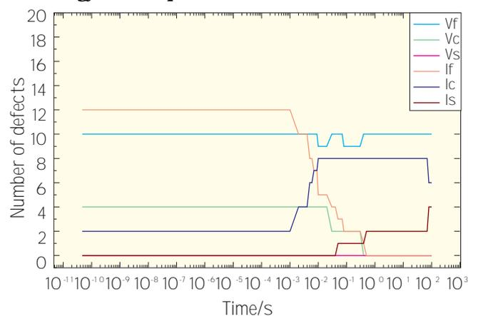
Fig. 6 – Isochronal annealing of the damage produced by a 3 keV PKA in Al at 75 K. Vf, If: free vacancies and interstitials; Vc, Ic: vacancy and interstitial clusters; Vs, Is: vacancies and interstitials arriving at the box surface
