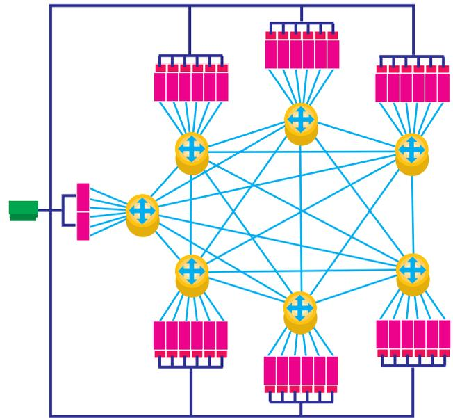
Fig.2 – The full connection between the 6 computational nodes and the integrated frontend at the left. The users will enter through the frontend computers
