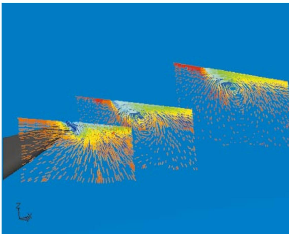
Vortex separation behind the transom of an IACC hull computed by FLUENT/UNS
