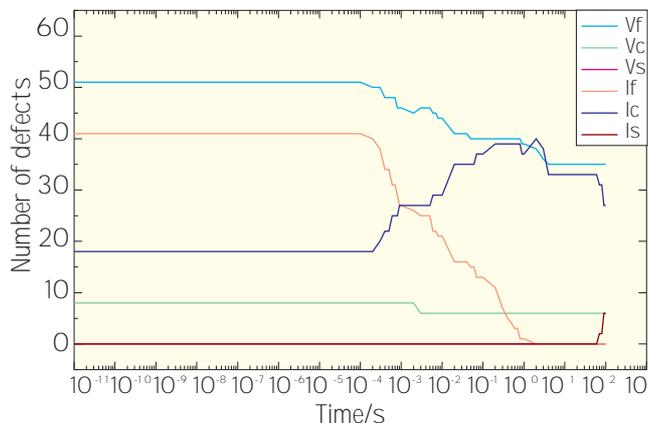
Fig.8 – Isochronal annealing of the damage produced by a 10 keV PKA in Al at 75 K. Legend as in fig. 6
