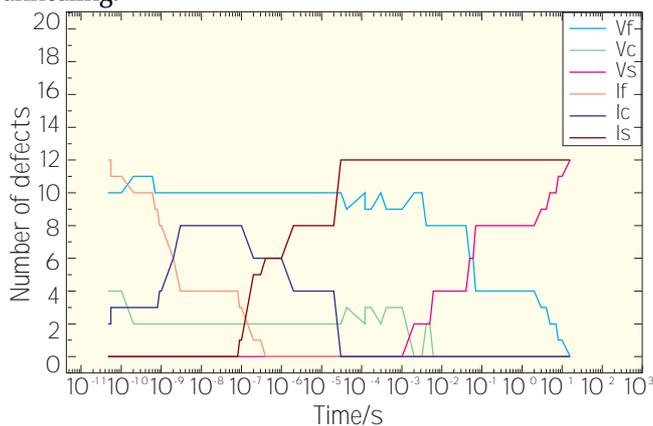
Fig. 7 – Isochronal annealing of the damage produced by a 3 keV PKA in Al at 300 K. Legend as in fig. 6
