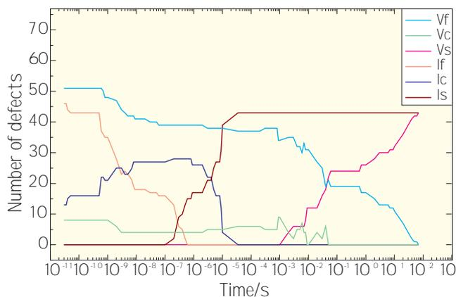
Fig. 9 – Isochronal annealing of the damage produced by a 10 keV PKA in Al at 300 K. Legend as in fig. 6
