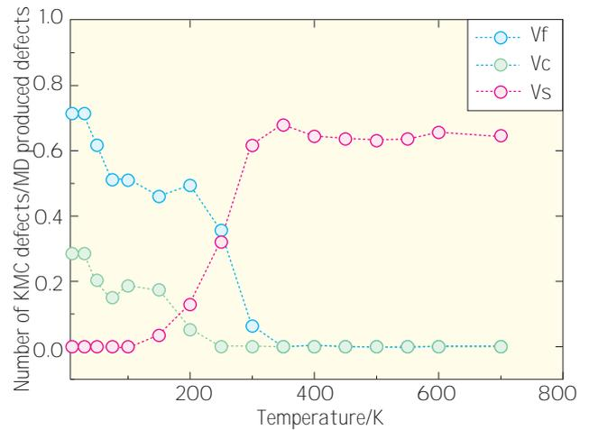
Fig. 11 – Annealing of vacancies produced by a 3 keV PKA in Al
