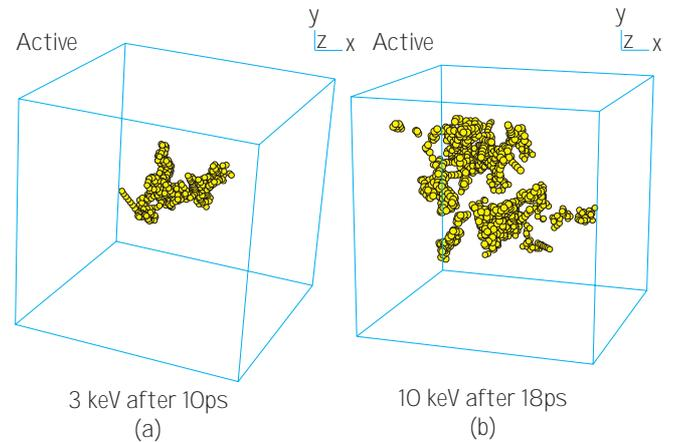
Fig. 3 – Displacement cascade produced by self ions of (a) 3 and (b) 10 keV in Al at 10 K
