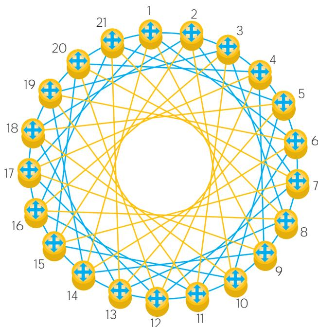
Fig. 3 – Swiss-T2 architecture with 21 (504 processors) nodes connected by a K-ring (K=3). Each of the vertices is a node with six quadri processor boxes connected by a crossbar.
