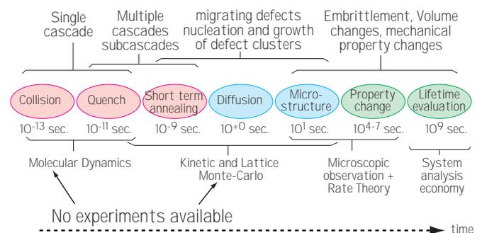
Fig. 1 – Radiation Damage evolution
