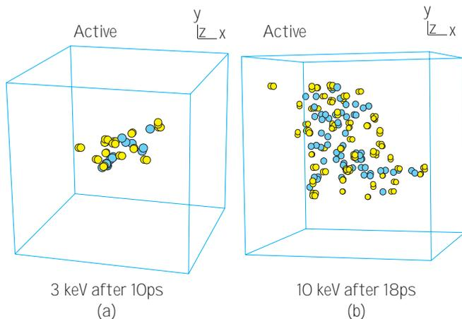
Fig. 2 – Defect distribution produced by self ions of (a) 3 and (b) 10 keV in Al at 10 K. Blue circles represent vacancies and the yellow ones interstitials
