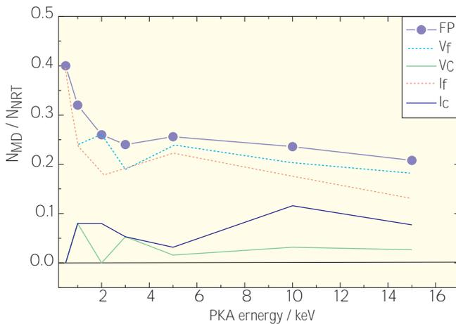
Fig. 5 – Relative amount of defects computed by MD in Al at 10 K ( $E_{th} = 16$  eV). FP: Frenkel pairs; Vf: free vacancies; Vc: vacancy clusters; If: free interstitials and Ic: interstitial clusters
