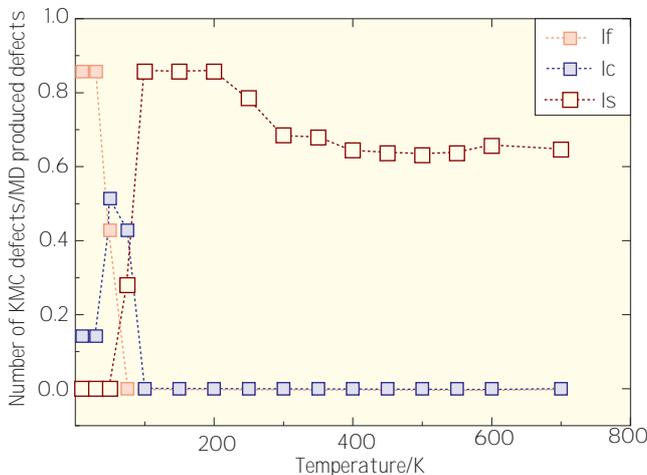
Fig. 10 – Annealing of interstitials produced by a 3 keV PKA in Al
