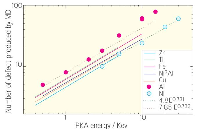
Fig.4 – Number of Frenkel pairs calculated with MD in Al at 10 K compared to values in other materials at 100 K, ref. [16]
